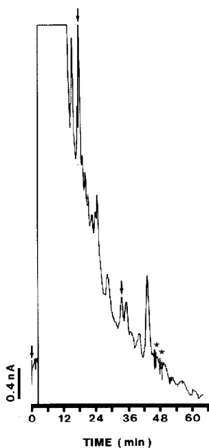
Fig. 1. Chromatogram of rat brain extracted with boiling acetic acid and processed through a metal-ligand affinity column and C_8 reversed-phase column. This type of chromatogram is representative of the results obtained for brain extracts processed without the use of CMS. The arrows above the peaks denote the positions of ME and LE. RFI is indicated by asterisks. Mobile phase, 128 ml of 50 mM potassium dihydrogenphosphate (adjusted to pH 2.3 with phosphoric acid)-29% acetonitrile, diluted to a final volume of 250 ml with LC water. Electrochemical detector, BAS LC-4B.
